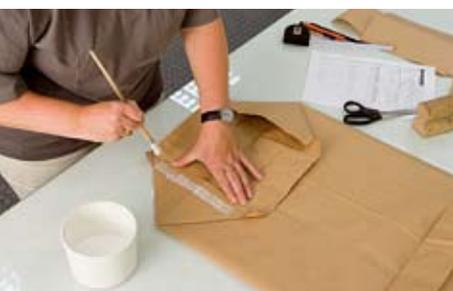
*Samples of the new designs are hand-made in our prototyping department. They are then tested on the original machines and further optimized, if necessary, before the bags go into full-scale production.*
